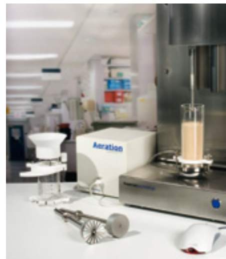
Figure 3: An “FT4” powder rheometer used to test wall friction between powders and surface coatings.
