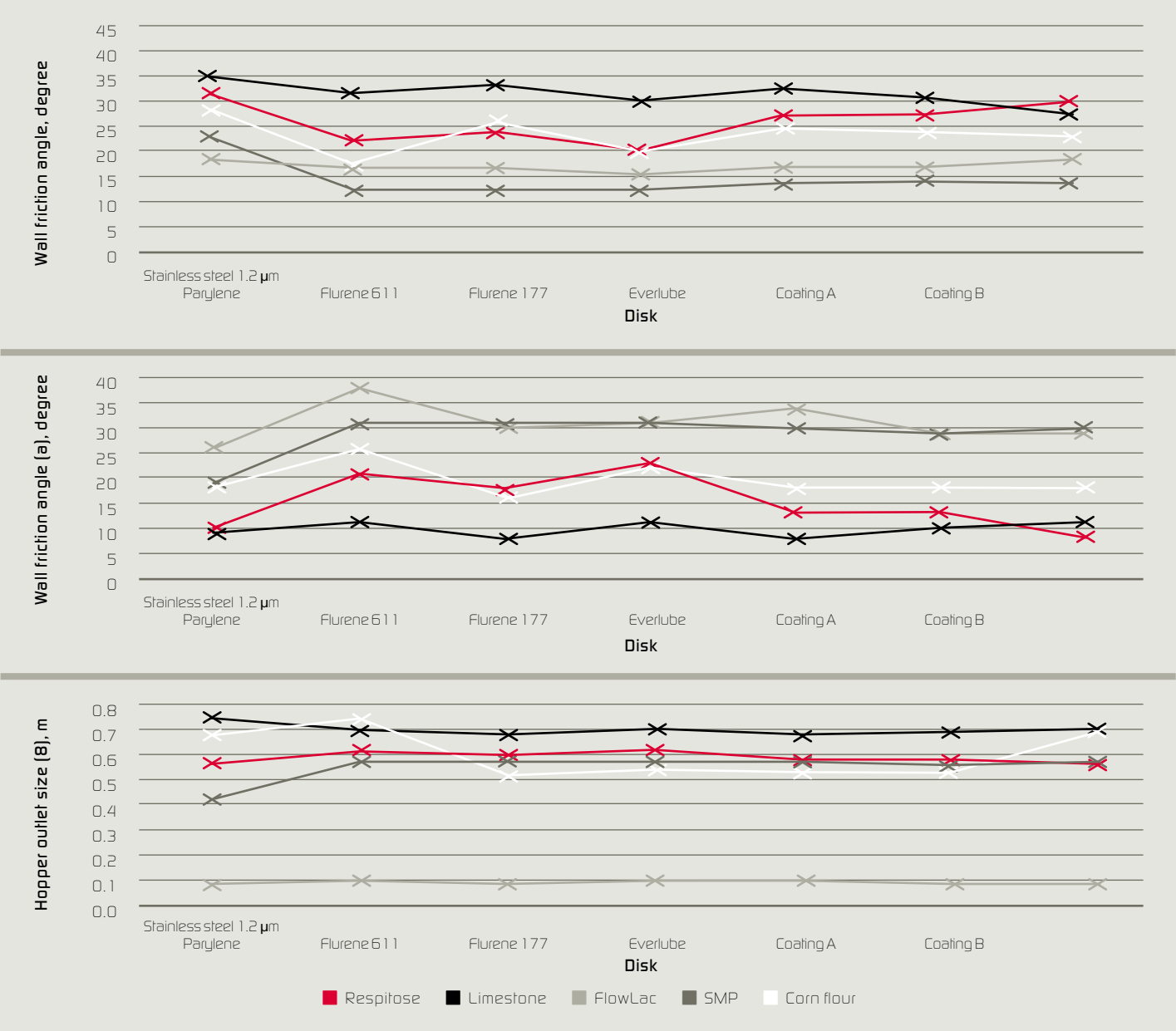
Figure 7: WFA, hopper half angle and outlet size indicate variations in performance for a range of coating/powder combinations.
